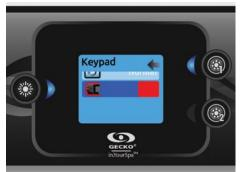
Note: With the in.k500 equipped with a selectable rim light color modul: If the "RGB backlight" option is enabled in the spa configuration an option will appear to allow selection of the keypad rim light color.
